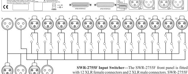
switchers are configured as input switchers. Each input switcher module connects any of 12 channels to the two analyzer input channels (A & B).
