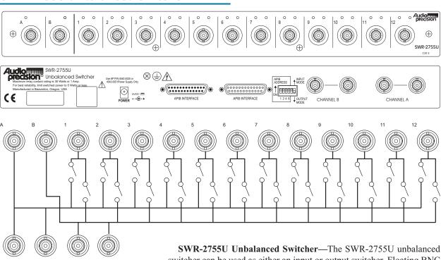
switcher can be used as either an input or output switcher. Floating BNC CHANNEL A CHANNEL B connectors help prevent ground loops. When used in the output mode, this REAR PANEL CONNECTORS
