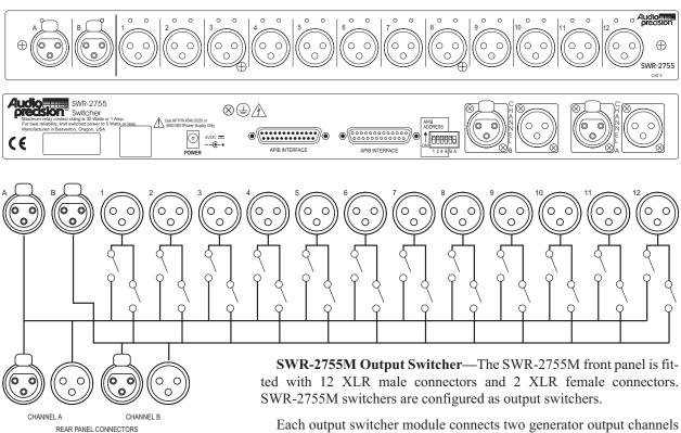
Each output switcher module connects two generator output channels (A & B) to any of 12 device input channels.
